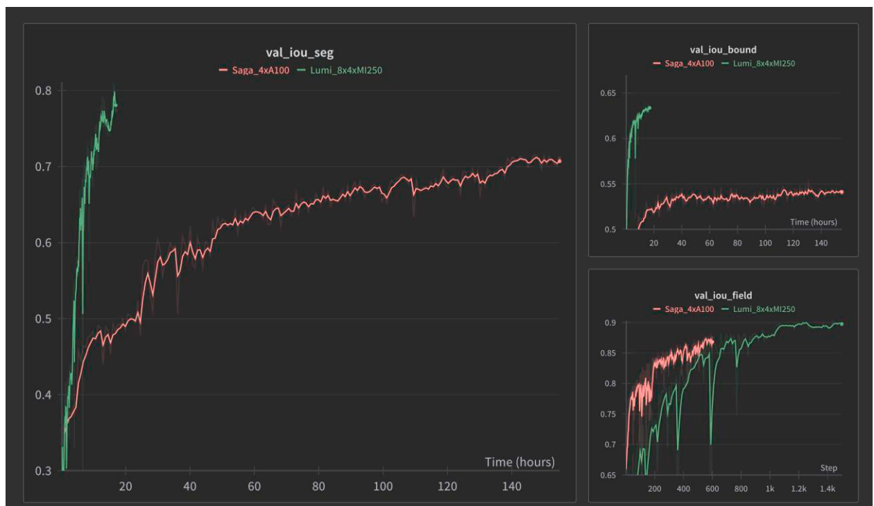
Figure 1. Comparison of model training performance on LUMI (green) vs. a conventional cloud HPC setup using NVIDIA A100s (red). (a) The val_iou_seg shows that the LUMI model achieves higher segmentation accuracy more quickly. (b) The val_iou_bound demonstrates superior boundary detection accuracy on LUMI. (c) The val_iou_field , our primary metric, stabilizes at \sim 0.94 on LUMI, a significant improvement over the A100 baseline.
